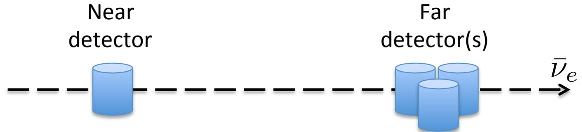
Oscillations are observed as a disappearance of  $\bar{\nu}_e$  in the far detector. Systematics are controlled by measuring the ratio of neutrinos in the far to the near detector.
